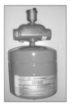
Liquid Solution Bypass Valve: The liquid solution bypass valve relieves system pressure from the liquid solution supply line to the return line as the system air handler controls are cycled off.
